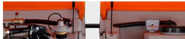
Dispensing hose with connection to first tank and switching valves
