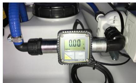
Meter FMT 3 with pulse output
